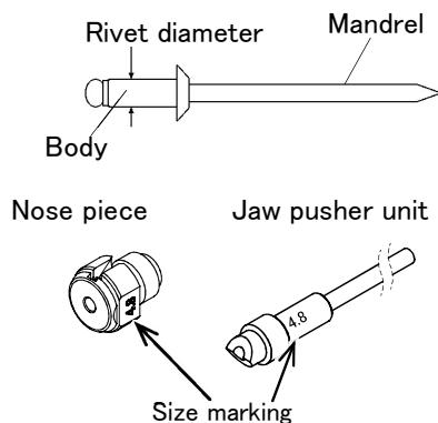
It is possible to use standard blind rivets in various sizes only by replacing the nose piece and jaw pusher unit.
