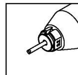
**9** If about half of the capacity of the mandrel collector is filled with mandrels, remove the mandrel collector and dispose of the mandrels contained in it.
