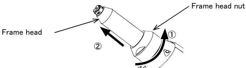
**3** Slide the detent ring until it contacts the rear (①), loosen and remove the jaw case head (② ·right screw).
